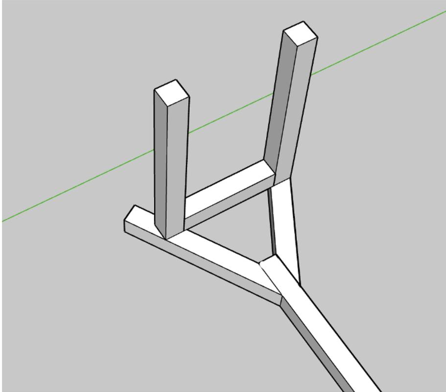
Trim the excess with a jigsaw. Once it is trimmed, the angles should be aligned correctly with the legs.
